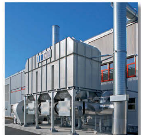
3-canister RTO system, size 20 000 m 3 n/h
